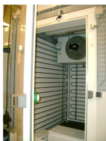
Figure 2. Styrofoam box in a cooling chamber used for cooling experiments with the agar cylinder.
