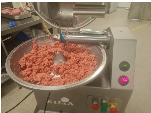
Figure 5. After the first mixing, samples were homogenised in a homogeniser shown in the figure.
