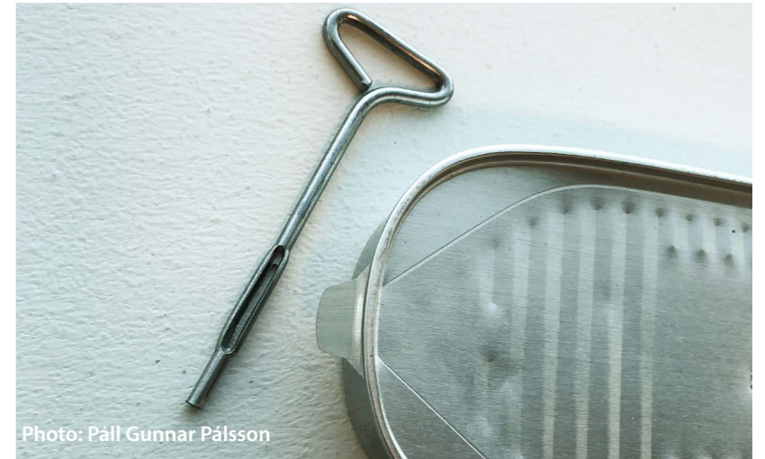
Can where a special key is included to open the can. At the tongue in which the key is placed, the material of the cover is quadrupled in the seam instead of being triple.
