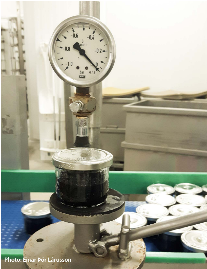
Facilities to measure the under-pressure in a jar with caviar, in this case the target is - 0.2 bars
