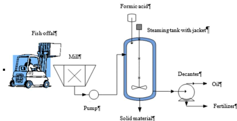
Figure 34. Typical processing line for production of liquid fertilizer from fish offal.
