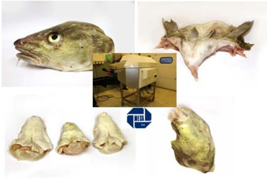
Figure 15. Production from Mesa 900 machine, upper right collar bone, down left tongues, down right cheeks.
