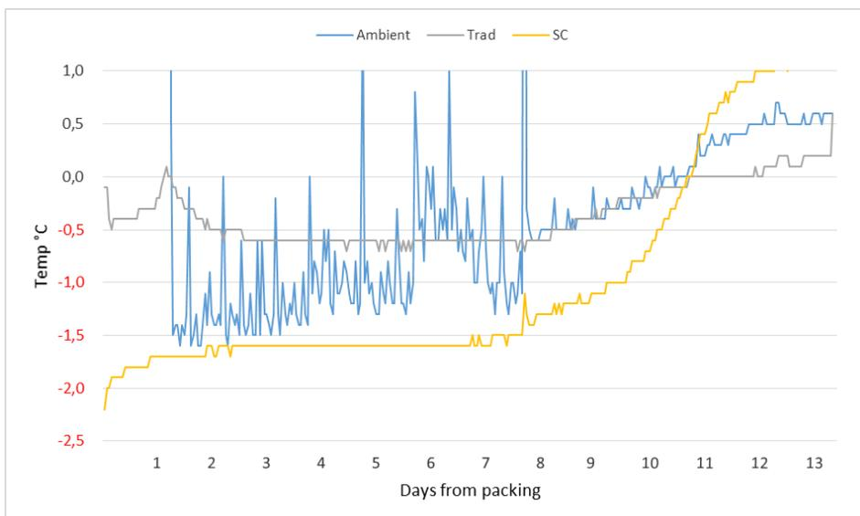
**Figure 22** Temperature profile from the boxes during transportation from Norway to Iceland and Matis cold room. (SC = Sub-chilled salmon; Trad = Salmon from traditional processing).
