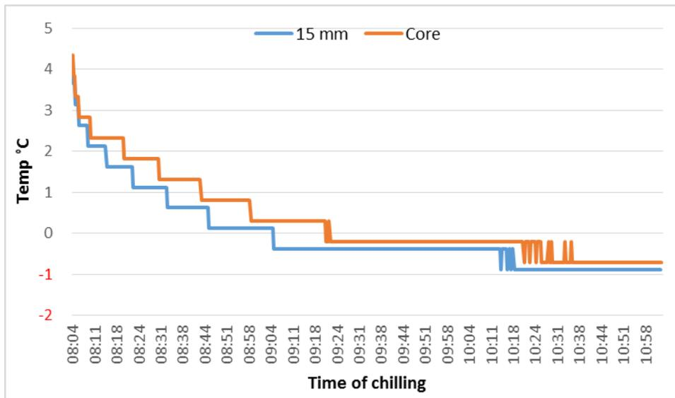
**Figure 7 Temperature profile during sub-chilling of salmon logging of sub-chilling for Hätälä.**
