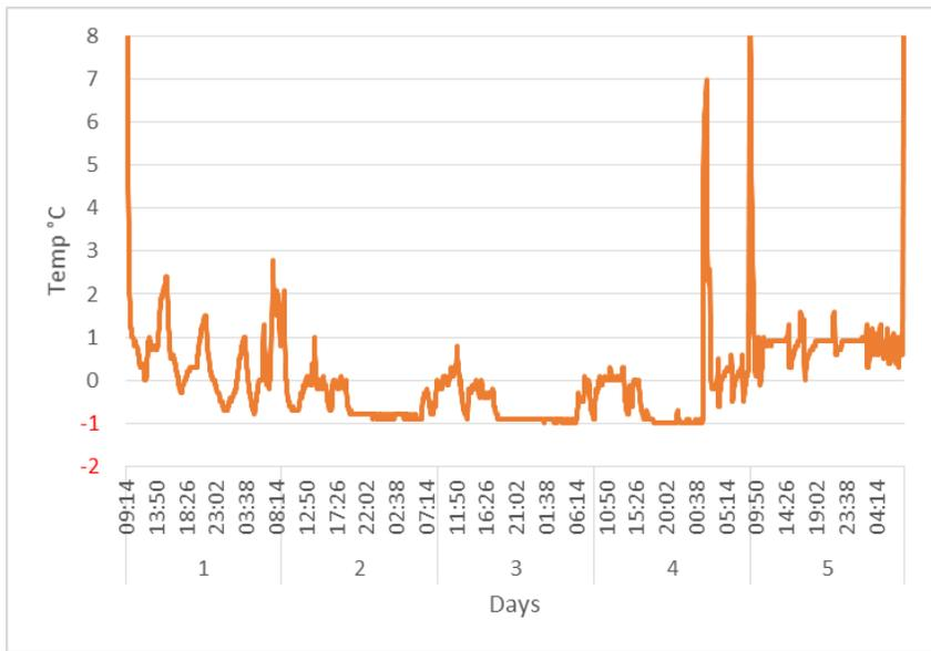
**Figure 27** Ambient temperature within the refrigerated truck during salmon shipment from Simanes in Norway to Norway Seafood in Denmark.
