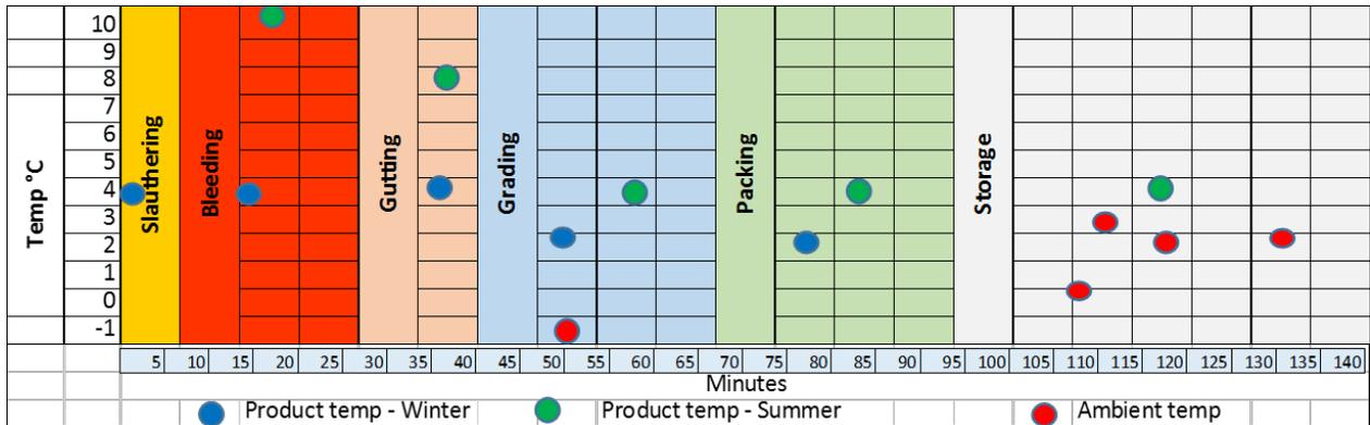
**Figure 23** Time and temperature during production in the Grieg Seafood Simanes factory during winter and summer time. Additionally, the temperature in the cold room was monitored from 15<sup>th</sup> of January to February 6<sup>th</sup> 2015.
