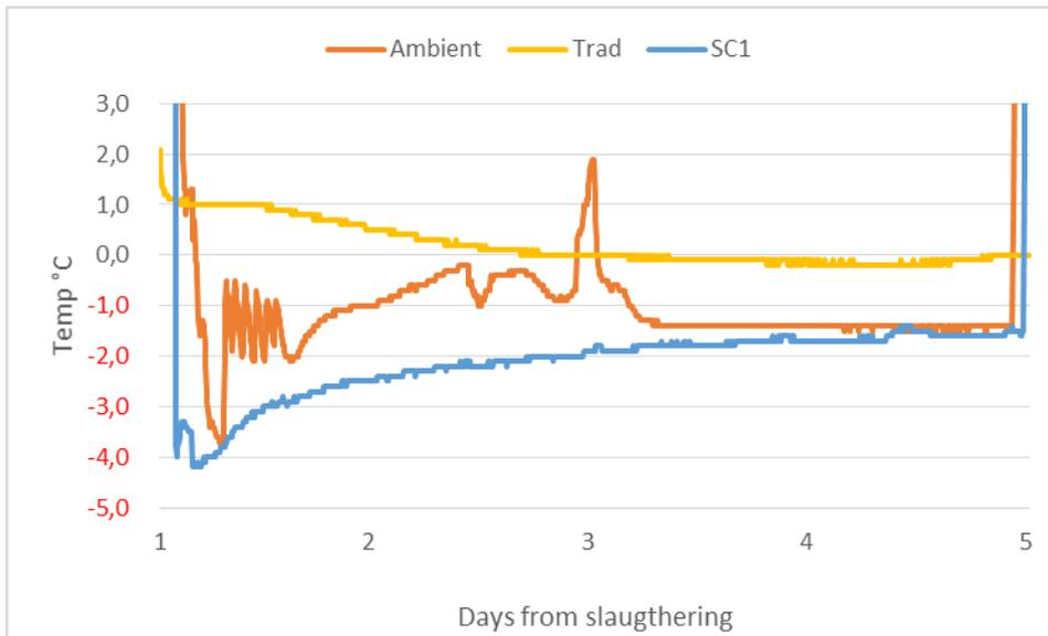
**Figure 25** Temperature profiles of sub-chilled salmon (SC1), traditional salmon (Trad) and ambient conditions during transportation from Simanes in Norway to logging on SC and traditional product and the ambient temp during transport to Saihoku Fisheries Corporation in Tokyo.
