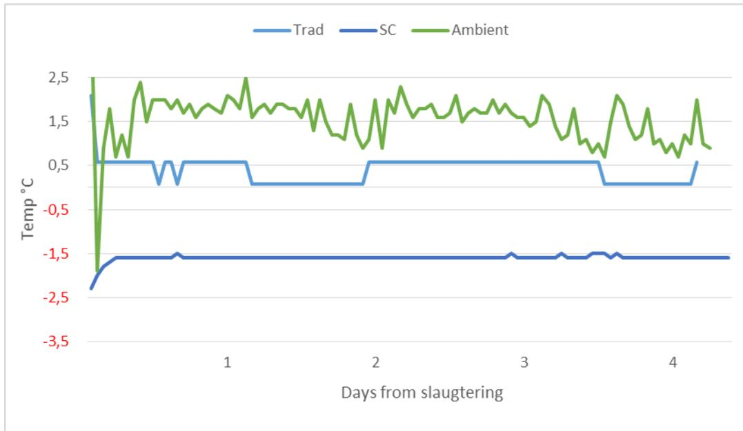
**Figure 11** The temperature profile in Hätälä of sub chilled salmon (SC), traditional salmon (Trad) and the cold room (ambient). The temperature of the sub-chilled salmon is steady around -1.5 °C and the traditional salmon around 0 °C.
