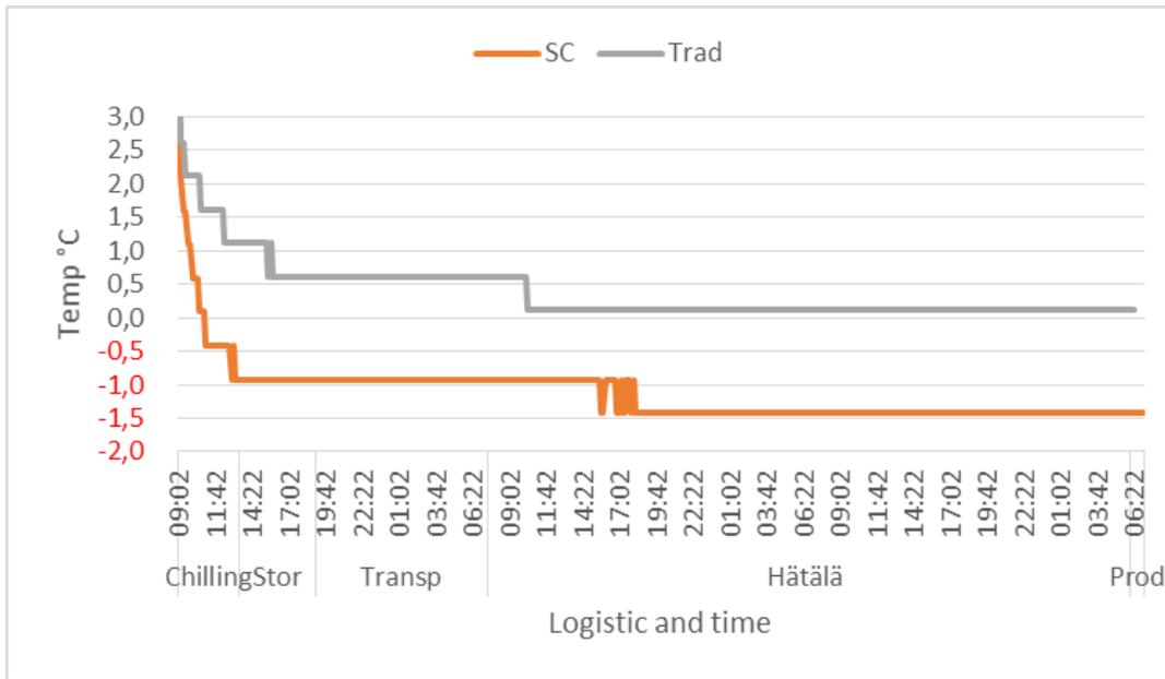
**Figure 10** The temperature profile of four days for the fish core during the sub-chilling process and transportation from Grieg Seafood in Norway to Hätäla in Finland. (SC = sub-chilled salmon; Trad = traditional salmon).
