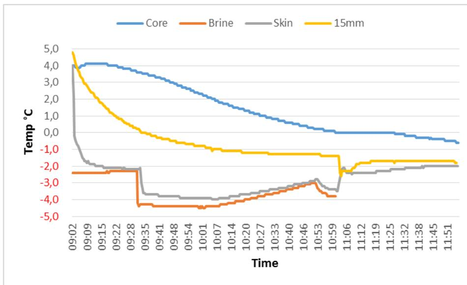
**Figure 8** The sub-chilling process of salmon at Grieg Seafood (Hätälä product March17<sup>th</sup>). The temperature was monitored in the brine, in the core of the fish, at 15 mm depth into the muscle, right under the skin.
