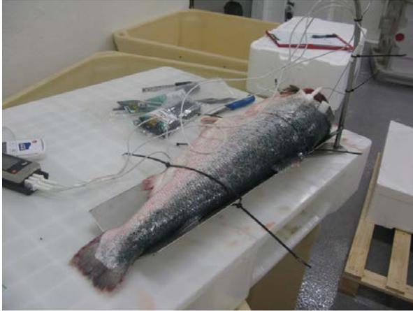
**Figure 2 Salmon with temperature sensors plugged.**
