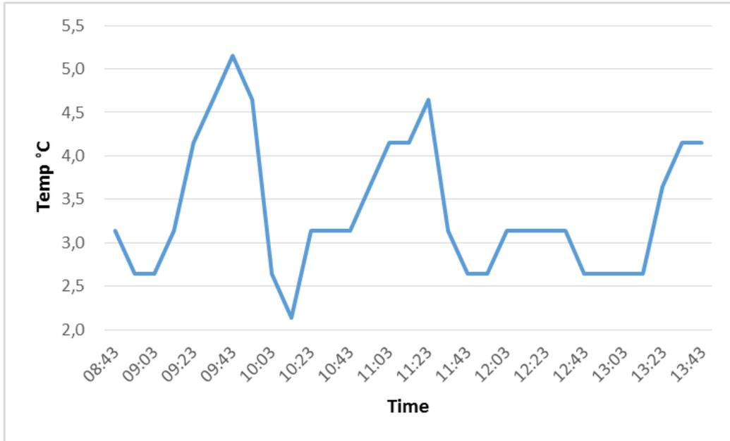
**Figure 5 Temperature profile of Grieg Seafood Simanes factory cold room.**
