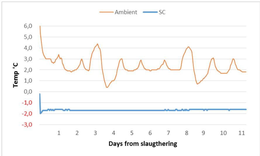
**Figure 26** Temperature profiles of sub-chilled salmon (SC) and ambient conditions during transportation from Simanes in Norway to Norway Seafood in Denmark by truck.
