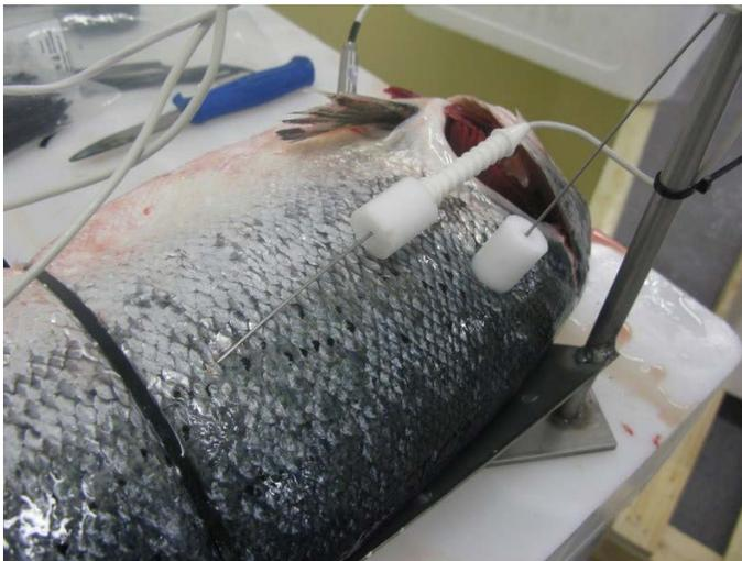
**Figure 4 Testor logger sensors placed in a salmon**
