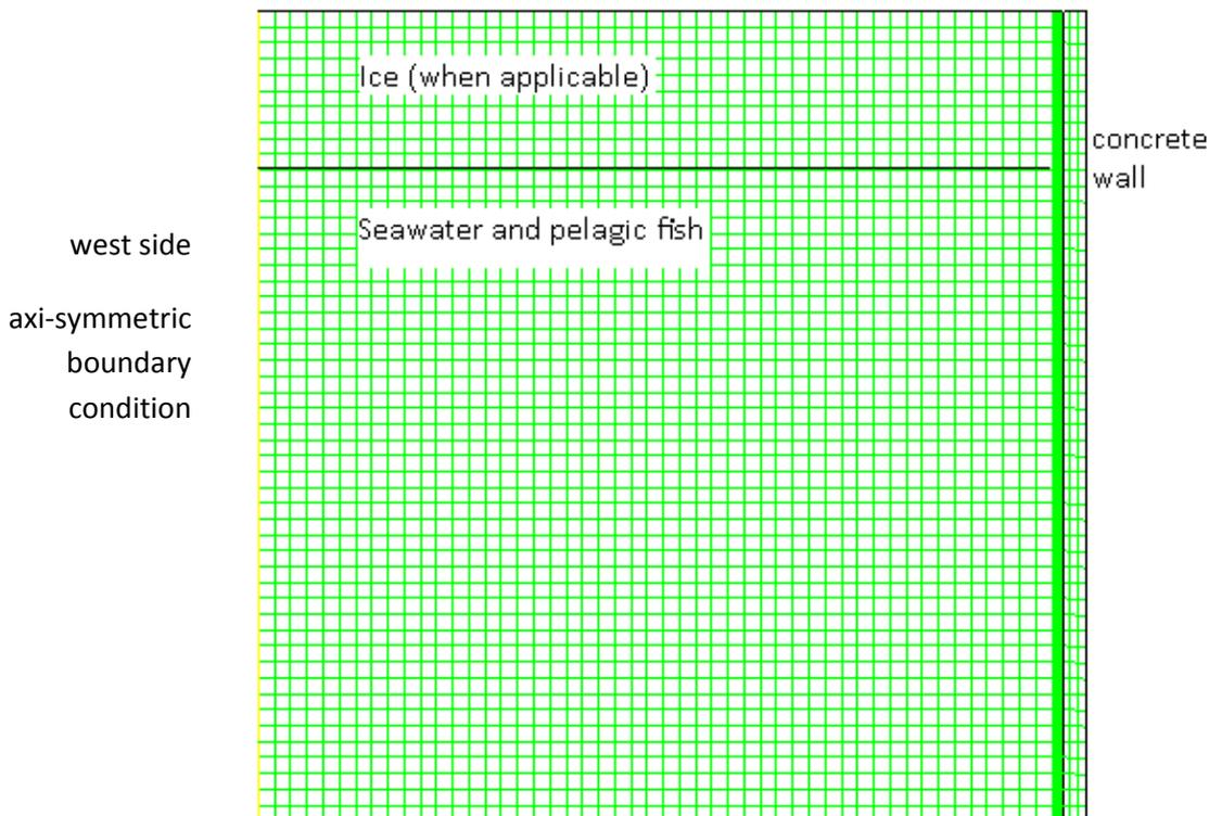
Figure 2: Meshing of the model, where an axi-symmetric boundary condition is used at the west side.
