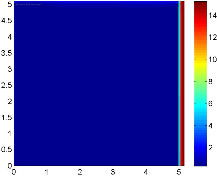
Figure 6: Temperature profile of the tank at 0.167h with a temperature load of 15°C applied.
