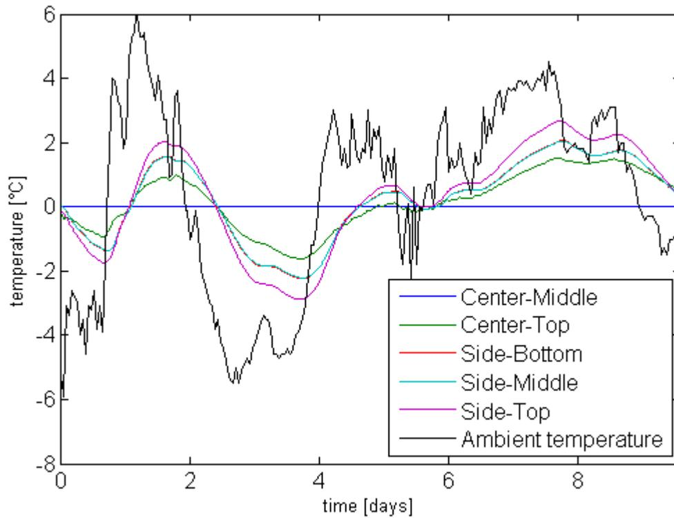
**Figure 5: Response of the system to an unsteady temperature load with no ice**
