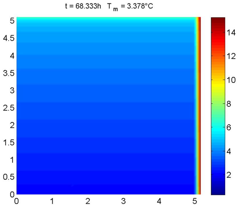
Figure 8: Temperature profile of the tank at 68.333h with a temperature load of 15°C applied.
