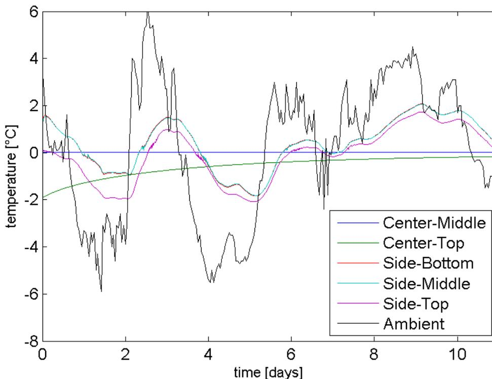
Figure 4: Response of the system to an unsteady temperature load with ice
