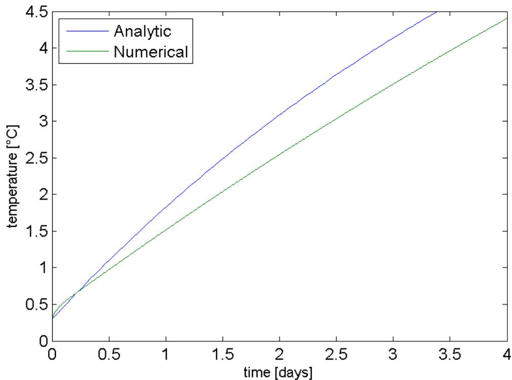
Figure 10: Comparison of an analytic method using lumped heat capacity system and the numerical method applied in other calculations.
