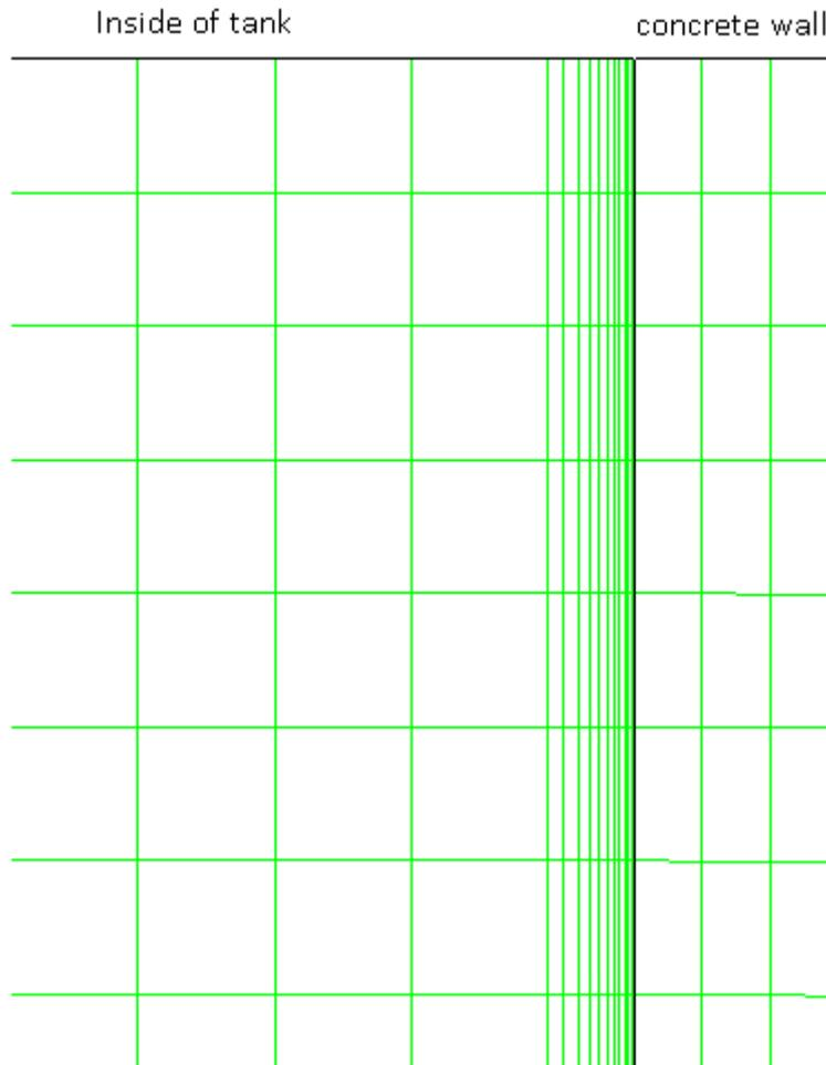
Figure 3: Meshing of the boundary layer at the concrete wall.
