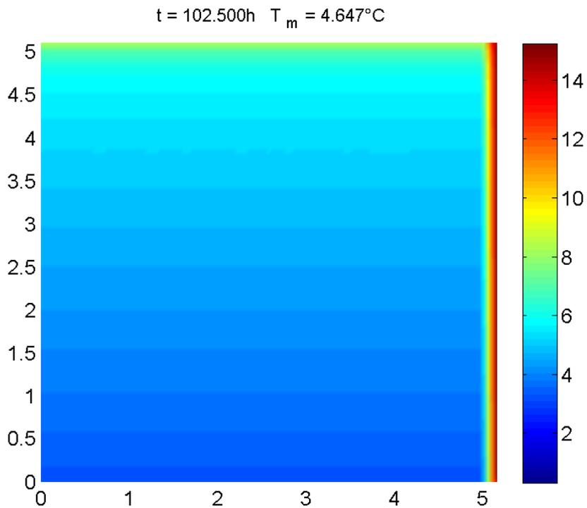
Figure 9: Temperature profile of the tank at 102.500h with a temperature load of 15°C applied.
