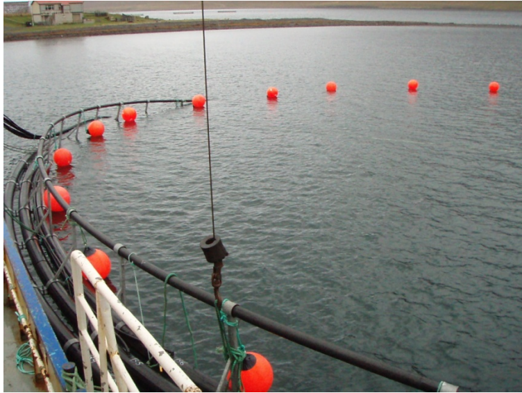
Figure 6 Sinking cage using crane and load
