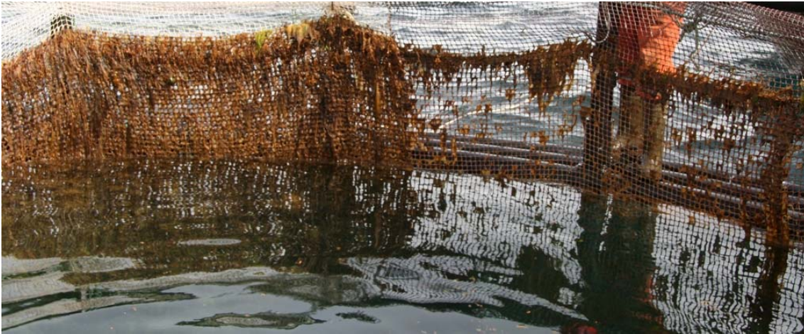
Figure 19. Net bag 2. On the left with side treated Byotrol and on the right with copper.
