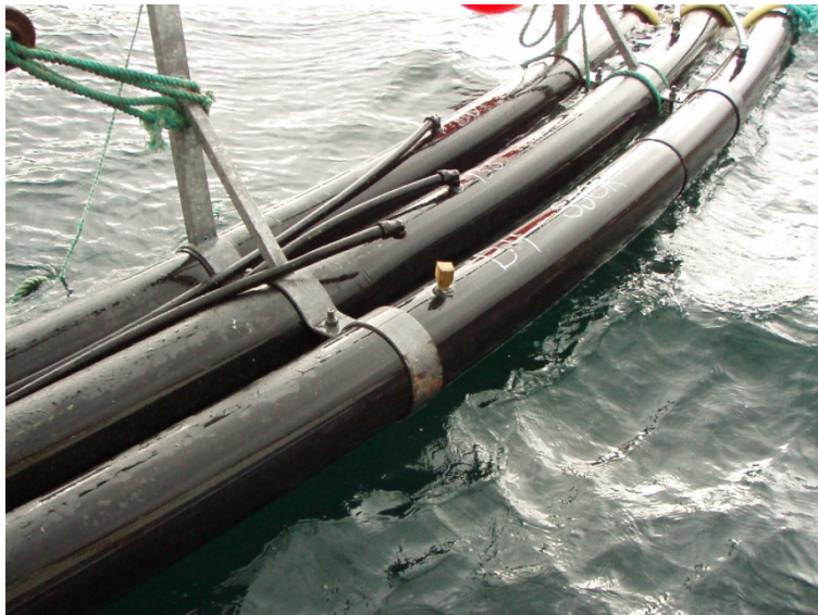
Figure 7 Broken valve, inlets and outlets can appear to be weak points in design if precaution is not taken while handling a cage
