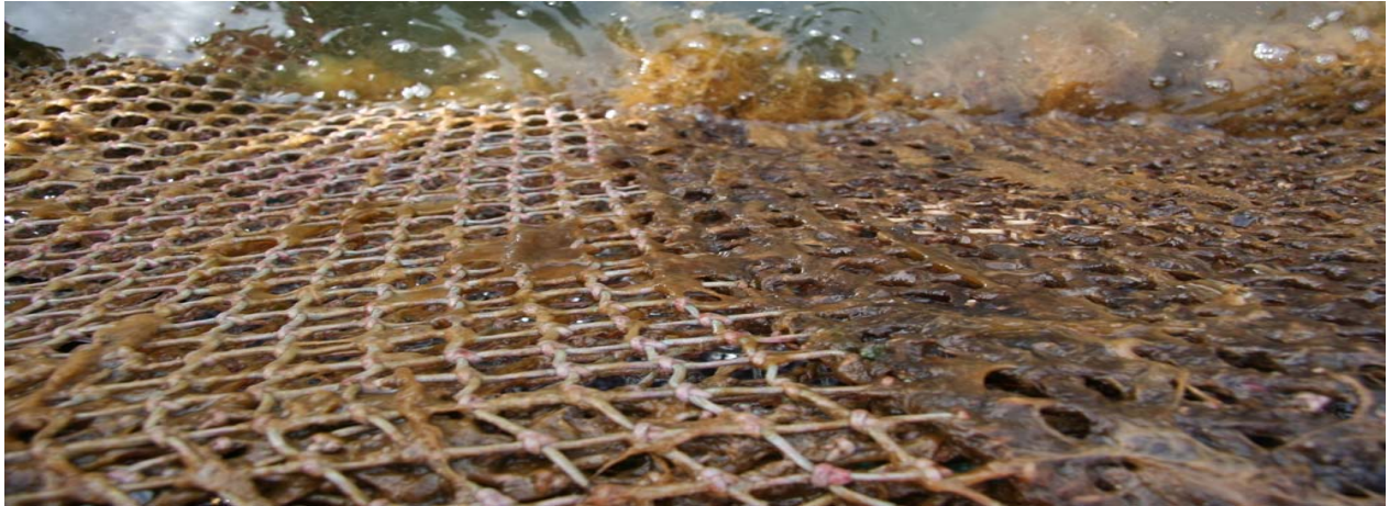
Figure 25. Net bag 2. On the left the bag is treated with Copper and on right with Byotrol.
